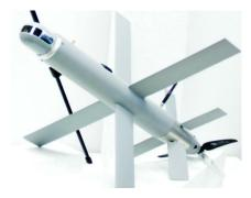
*Hero-30*, formerly WASP (UVision) is presented as a mini ISR UAV and not as a loitering munition, however it has all the attributes of being a very successful and effective LM. Its shape with cruciform wings is highly manoeuvrable and perfectly adapted to attacks from all angles, it loiters for 30 minutes, it has a data link range of 10 km, it can carry a 2.2-pound payload, it weighs 6.5 pounds, and is launched from a launch canister (all eight wings are foldable).
